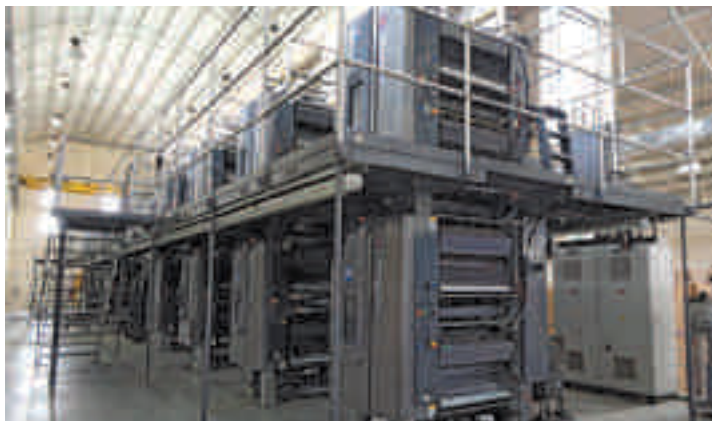
The new Goss Magnum press enables the Vision Group to print 64 full-color pages in one pass.
